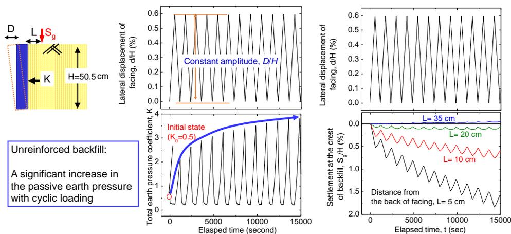
Figure 20. Settlement in dense air-dried Toyoura sand ( $D_r = 90\%$ ) and an increase in the passive earth pressure on the back of the facing by cyclic lateral displacements at the top of the FHR facing in a small model test (Tatsuoka et al., 2009, 2010b).
