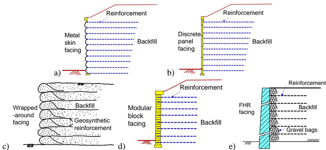
Figure 9. Different combinations of facing and reinforcement (refer to Table 1).
