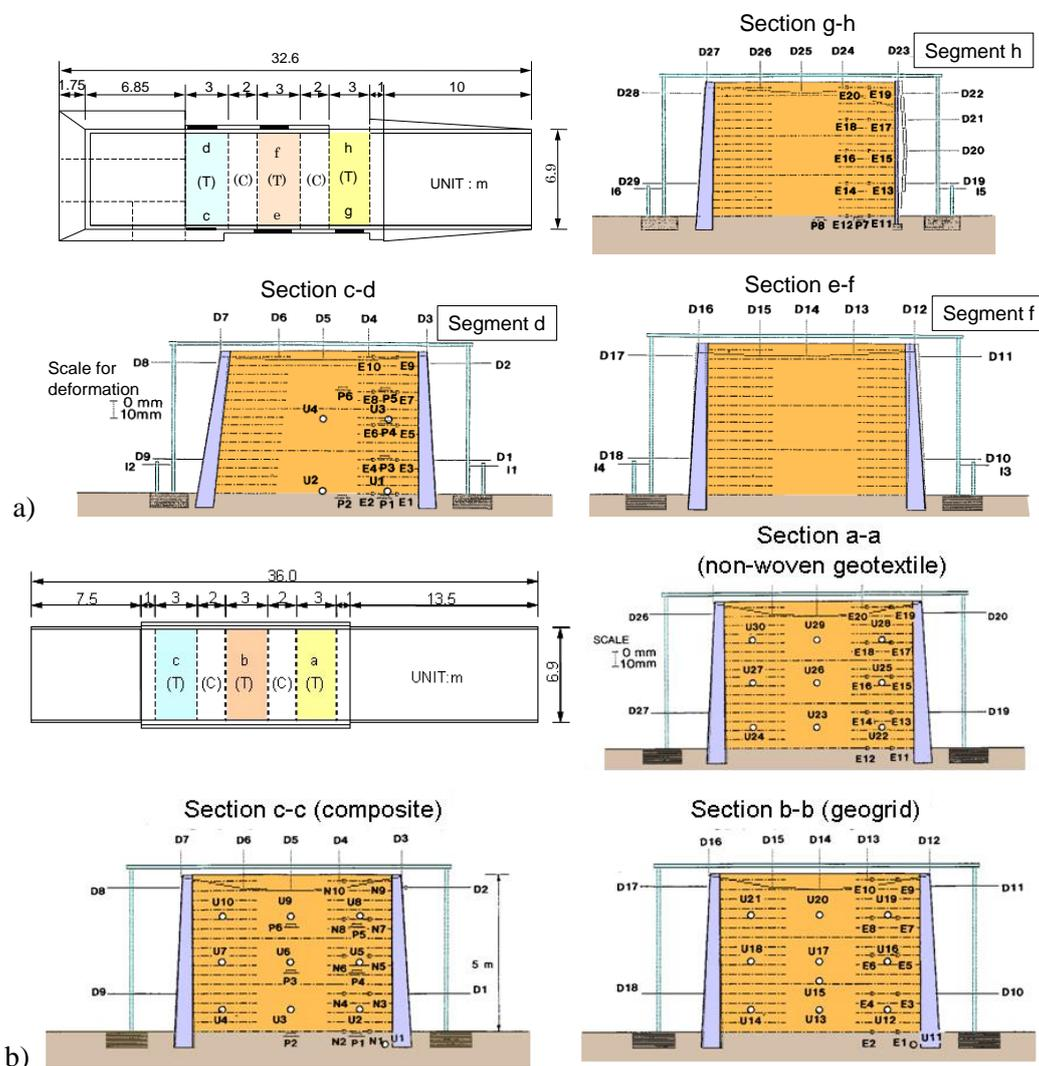
Figure 7. Plan and cross-sections two years after wall construction: a) JR No. 1 test embankment with sand backfill; and b) JR No. 2 test embankment with clayey soil backfill (Tatsuoka et al., 1990, 2000, 2008).
