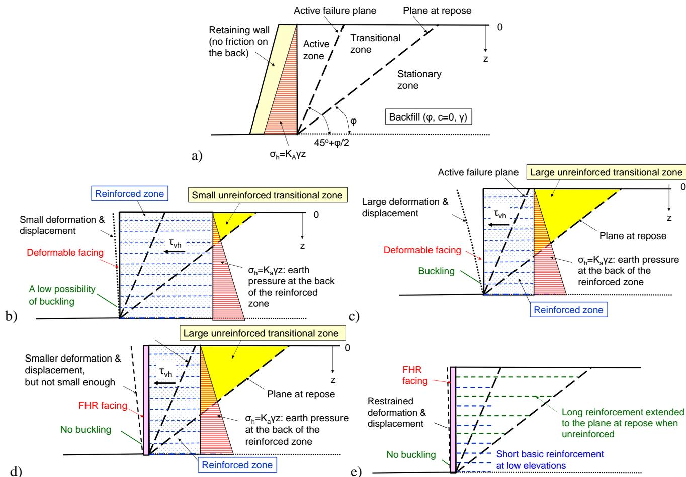
Figure 13. Active failure mechanism: a) conventional cantilever RW; and reinforced soil RWs with: b) flexible facing & long reinforcement; c) flexible facing & short reinforcement; d) FHR facing & short reinforcement; and d) FHR facing & several long reinforcement layers and short reinforcement layers at low elevations.
