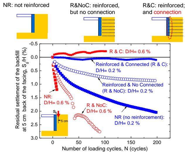
Figure 25. Settlement at 5 cm back of the FHR facing in the backfill of dense air-dried Toyoura sand ( $D_r= 90\%$ ) by cyclic lateral displacement at the top of FHR facing with a height  $H= 50.5$  cm hinged at the bottom in three model walls (see Fig. 20 for the details of the model tests) (Tatsuoka et al., 2009, 2010b).
