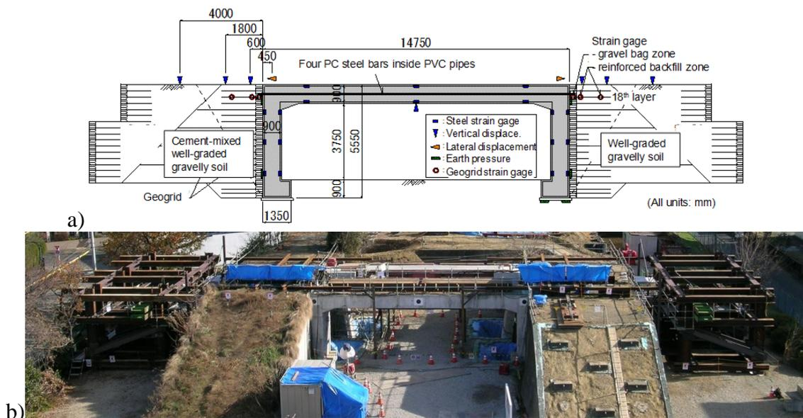
Figure 24. a) Full-scale model of GRS Integral Bridge at Railway Technical Research Institute; and b) view during lateral cyclic loading tests (Koda et al., 2013; Tatsuoka et al., 2016).
