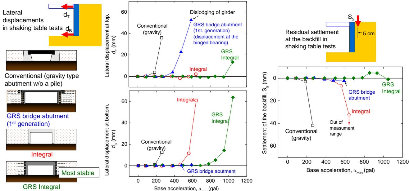
Figure 26. Residual lateral displacements at the top and bottom of the FHR facing and residual settlement at 5 cm back of the facing in shaking table tests of four bridge models ( $\alpha_{max}$ : the amplitude of input acceleration at a frequency of 5 Hz) (Tatsuoka et al., 2009).
