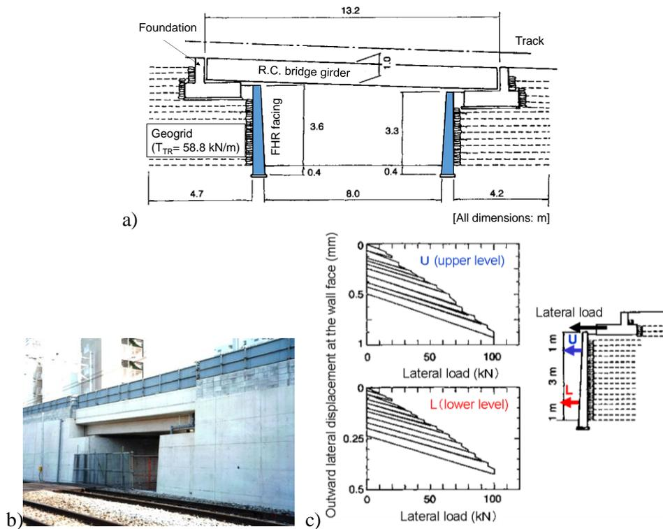
Figure 21. GRS Bridge Abutments (first generation) near Sakuradai station, Seibu Ikebukuro line, Tokyo; a) elevation of the bridge; b) completed bridge; and c) lateral loading test of a GRS Bridge Abutment (other than those shown in Figs. a & b), performed 24 June 1993.
