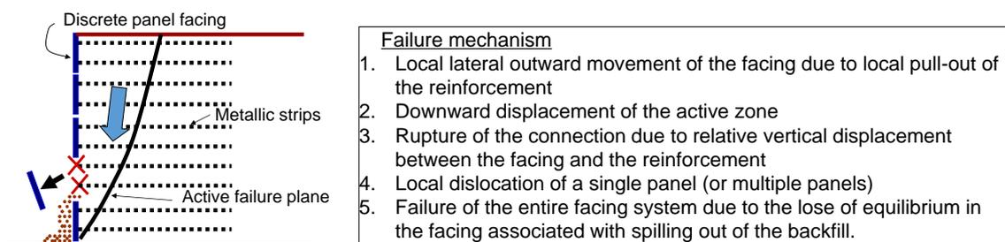
Figure 16. A typical failure mode of steel strip-reinforced soil RW having a discrete panel facing.
