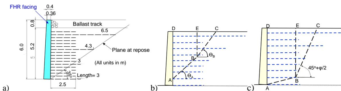
Figure 14. a) Typical GRS RW with FHR facing designed following the current design code; and two-wedge stability analysis: b) general; and c) most likely critical failure planes when the facing is FHR.
