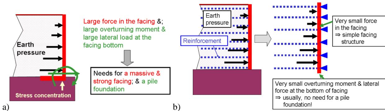
Figure 10. a) Disadvantages of conventional type cantilever RW; and b) advantages of GRS RW with FHR facing as a continuous beam supported at many points (Tatsuoka, 1993; Tatsuoka et al., 1997b).
