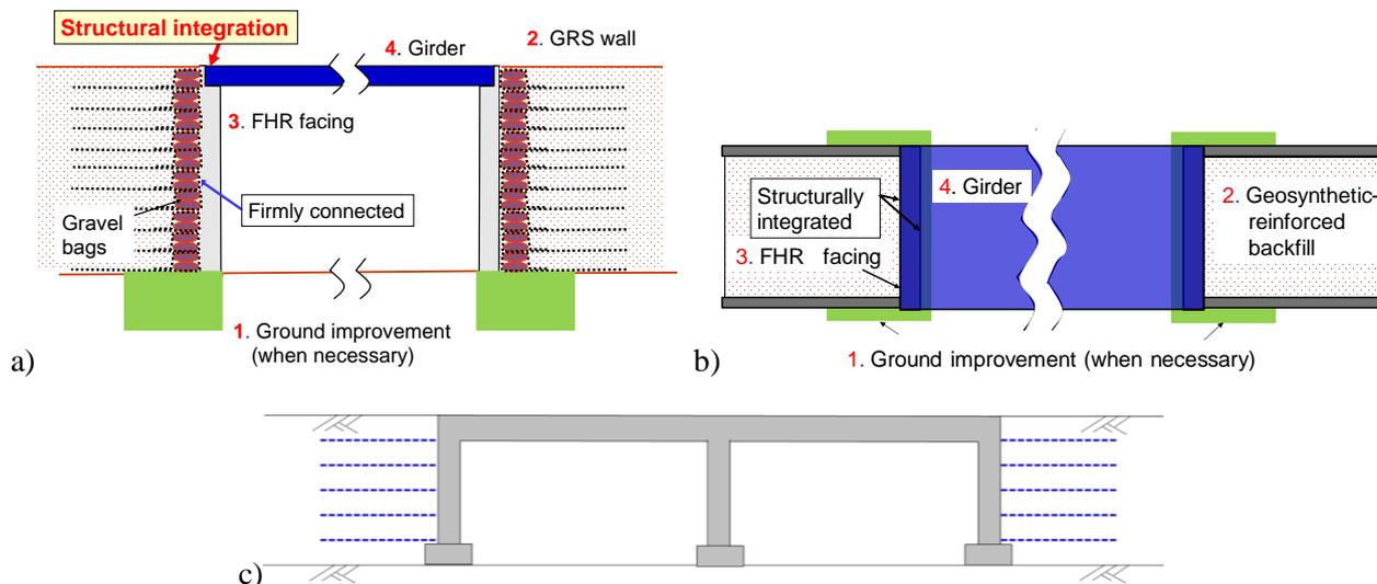
Figure 3. GRS Integral Bridge: a) elevation; b) plan; and c) a long-span girder vertically supported by a pier at its center (Tatsuoka et al., 2009, 2014, 2015, 2016).
