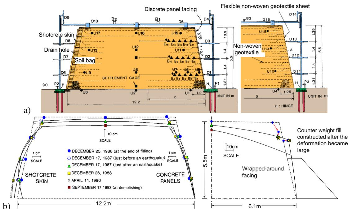
Figure 6. Chiba No. 3 embankment: a) cross-sections at the center and at the rear side; and b) deformation of the cross-sections at the center and at the rear side (Tatsuoka et al., 1990, 2000, 2008).
