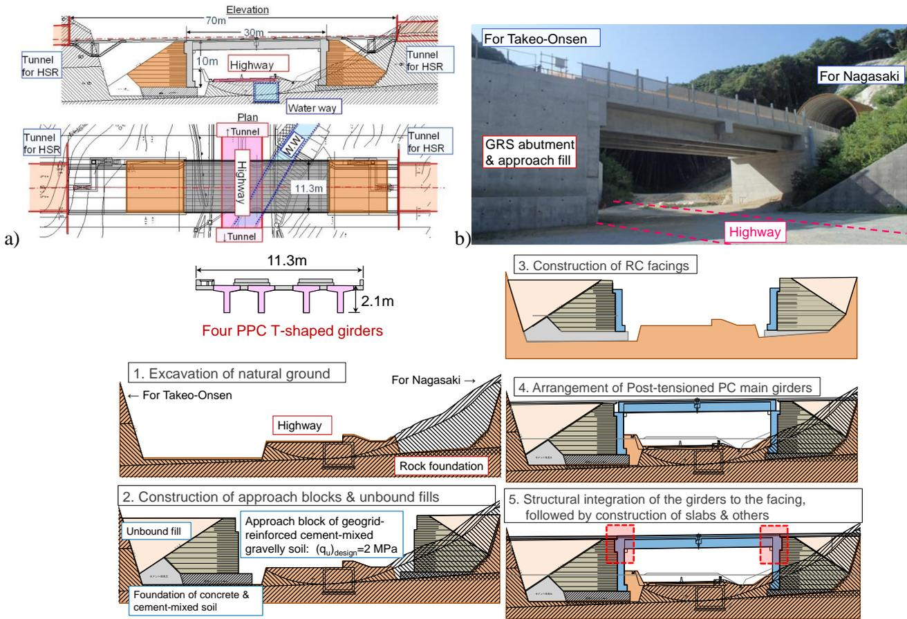
Figure 28. GRS Integral Bridge at Genshu, Nishi-Nagasaki Route, Kyushu Shin-kan-sen: a) structure; b) completed bridge; c) cross-section and construction procedure (Soga et al., 2018).
