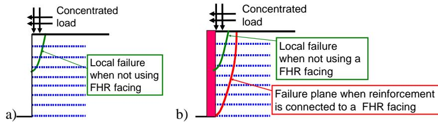
Figure 17. Failure of reinforced soil RW when subjected to concentrated load near the wall face at the crest of wall: a) deformable facing; and b) FHR facing connected to reinforcement layers.
