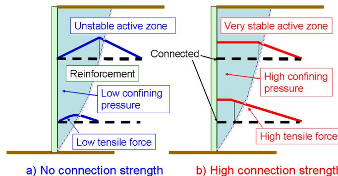
Figure 11. Different wall behaviours: a) no connection force between the reinforcement and the facing; and b) high connection force (Tatsuoka, 1992).
