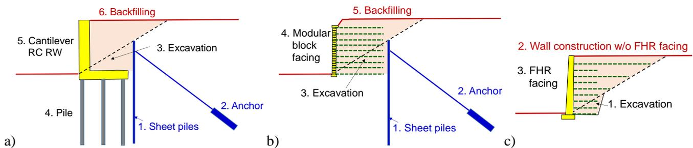
Figure 15. Construction of RW on slope: a) conventional cantilever RC RW; b) reinforced soil RW with relatively long reinforcement; and c) GRS RW having FHR facing with several long geogrid layers at high elevations and short geogrid layers at low elevations (Tatsuoka et al., 1997b). Note: Numbers refer to construction stage.
