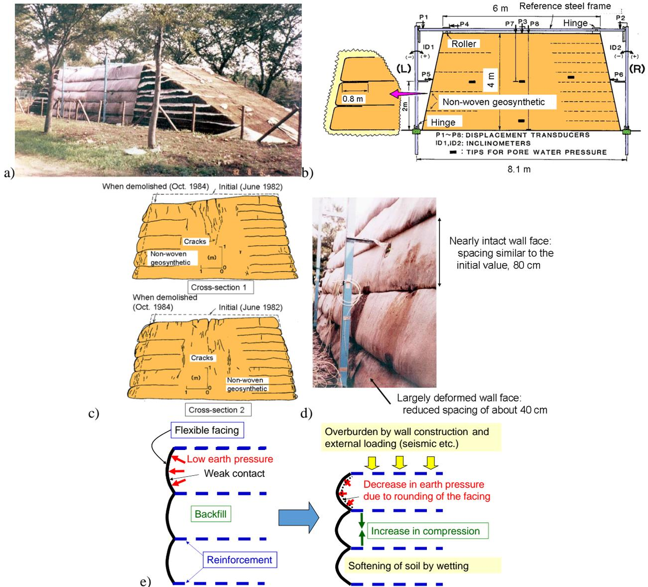
Figure 4. Chiba No. 1 embankment of clayey soil (Tatsuoka & Yamauchi, 1986; Tatsuoka et al., 1990, 2000, 2008): a) immediately after completion; b) initial cross-section; c) cross-section exposed when demolished (about two years later after the construction); d) wall face after large deformation at the bottom of the wall by several heavy rainfalls; and e) mechanism of the development of large deformation at flexible wall face.
