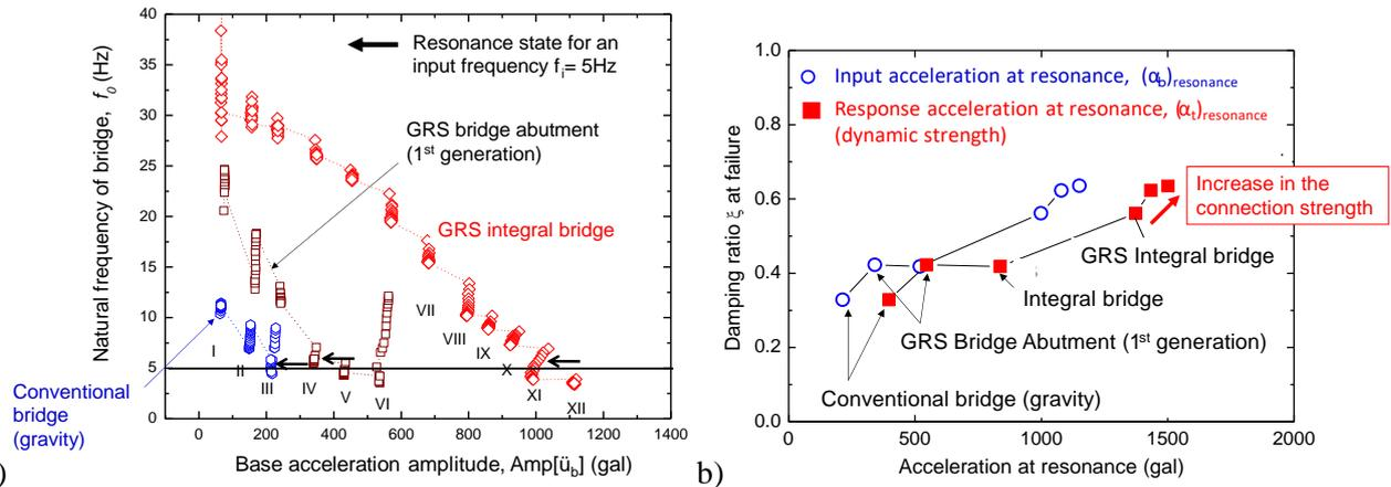
Figure 27. a) Decrease in the natural frequency  $f_0$  with an increase in the input acceleration at a frequency equal to 5 Hz; and b) damping ratio plotted against input acceleration and response acceleration at resonance of different bridge models in the shaking table tests described in Fig. 26 (Munoz et al., 2012).
