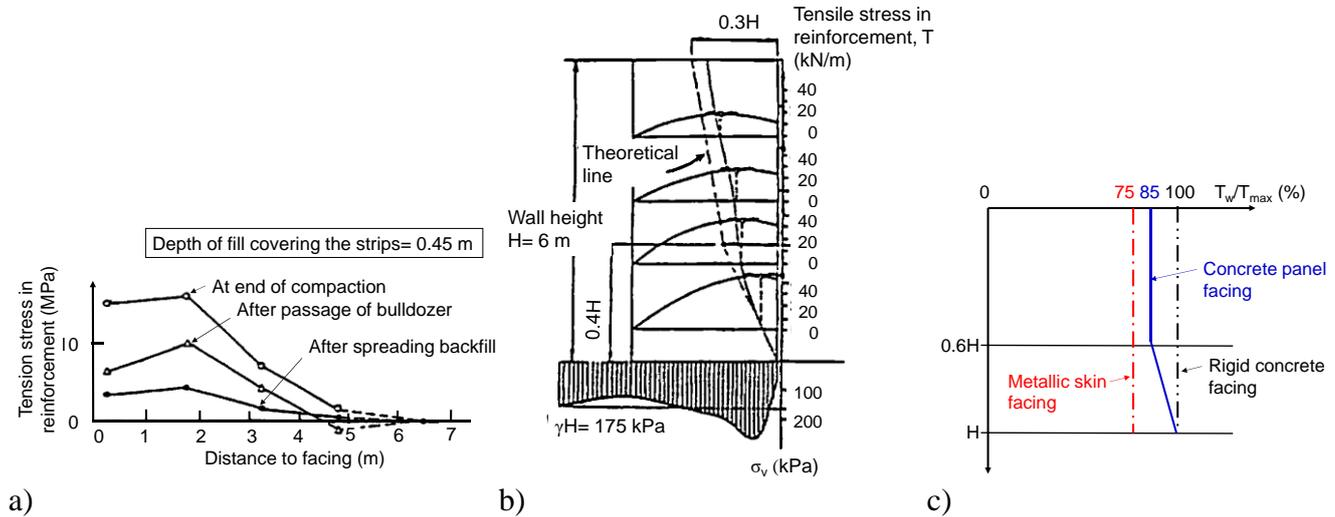
Figure 12. Distribution of tensile forces along reinforcement for Terre Armée RWs: a) measured during backfilling; b) measured in a test wall ( $H=6\text{ m}$ ); c) the effect of facing rigidity by FEM analysis (Schlosser, 1990).
