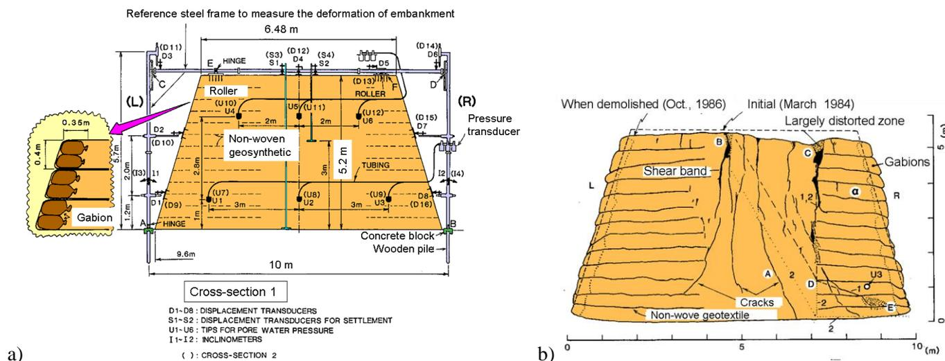
Figure 5. Cross-sections of Chiba No. 2 embankment: a) when completed; and b) one year after an artificial heavy rainfall test (Tatsuoka & Yamauchi, 1986; Tatsuoka et al., 1990, 2000, 2008).
