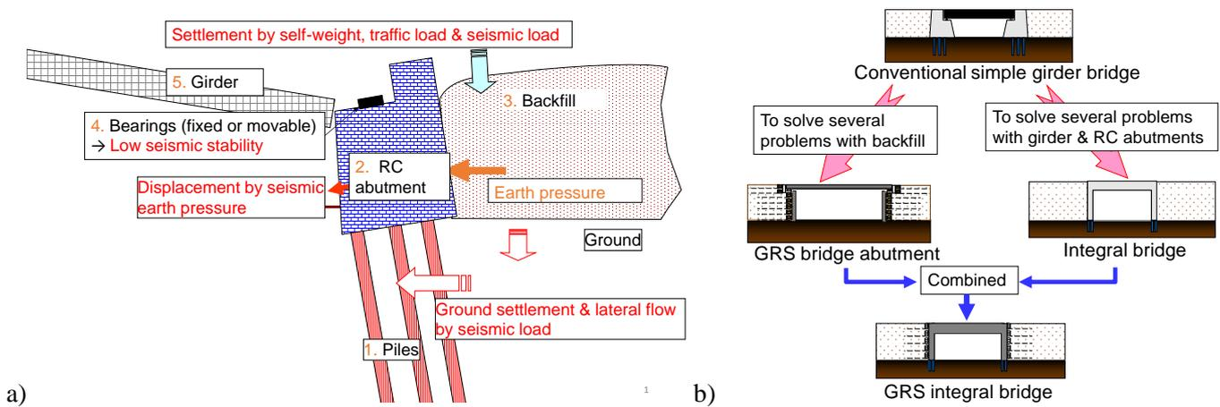
Figure 19. a) Typical serious problems with conventional type simple girder bridge; and b) development towards GRS Integral Bridge (Tatsuoka et al., 2009, 2016).
