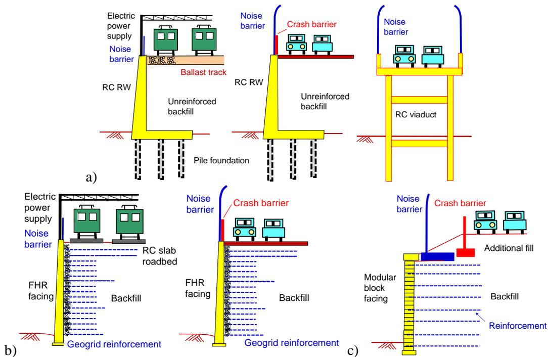
Figure 18. Typical elevated structures: a) conventional (piled cantilever RC RW & RC viaduct); b) GRS RW with FHR facing; and c) reinforced soil RW with modular block facing.
