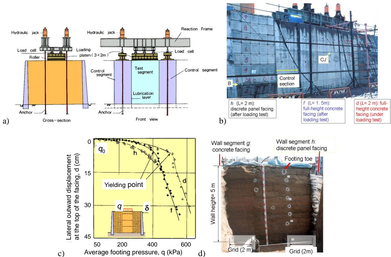
Figure 8. Vertical loading test of JR No. 1 sand embankment (Tatsuoka et al., 1990, 2000, 2008): a) loading method; b) view of wall segments  $d$ ,  $f$  and  $h$  after loading test; c) lateral displacement at the facing top vs. footing load relations of wall segments  $d$ ,  $f$  and  $h$  ( $q_0$  = average pressure due to the weight of loading apparatus); and d) shear bands observed in segment  $h$  (having discrete panel facing).
