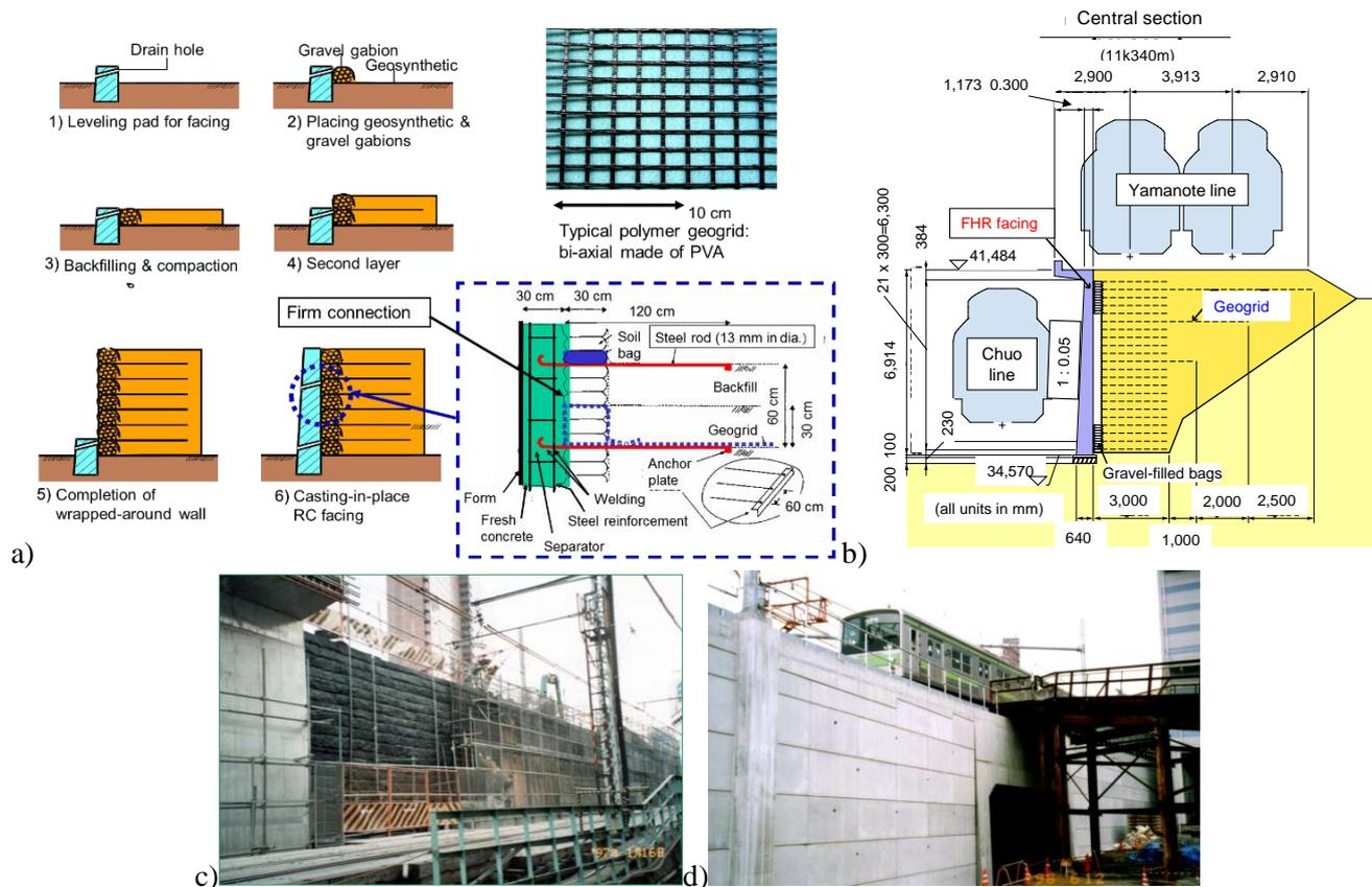
Figure 1. a) Staged-construction of GRS RW with FHR facing; and a typical wall near Shinjuku Station, Tokyo, constructed during 1995 – 2000: b) cross-section; and c) & d) views during construction and completed.
